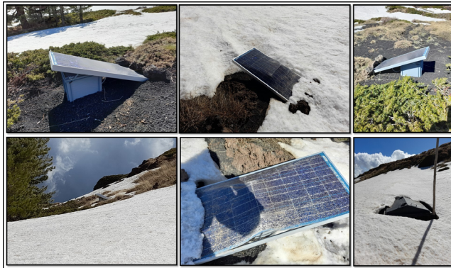
Figure 8 Images of the stations under the snow during the array decommissioning at the end of March 2022. The two central photos show the solar panel (CONC5 station) damaged by the snow load during the winter.
