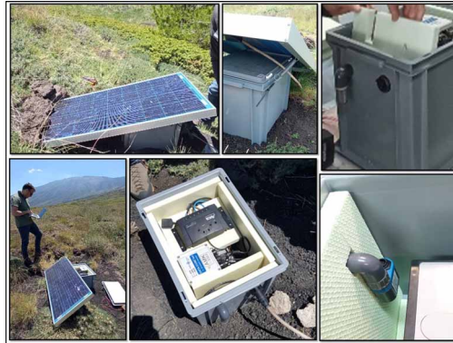
Figure 7 Images of the custom-made housing for instrument deployment. Note the housing thermal insulation and spring anchoring system of the solar panels to the box.
